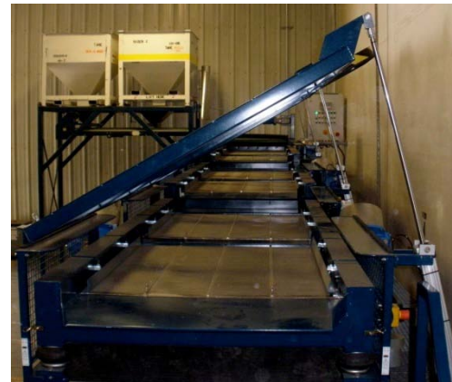
Photo: Three flat screen sizers placed in line / seed supply by 90° supply belt
