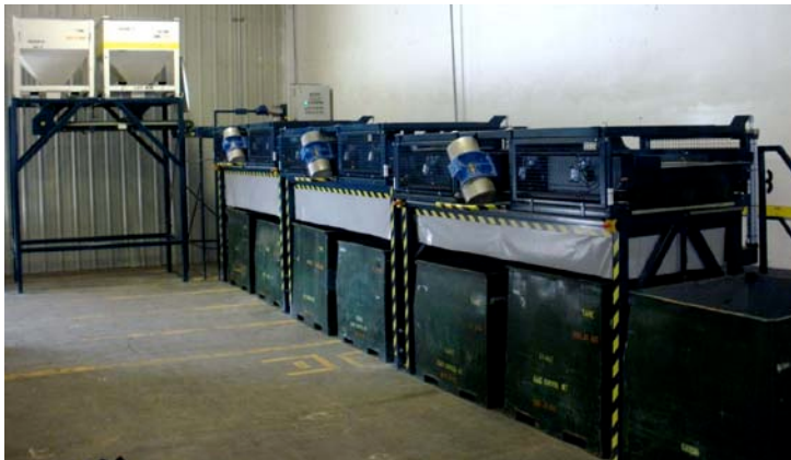
Photo: Three flat screen sizers placed in line / seed supply by 90° supply belt
