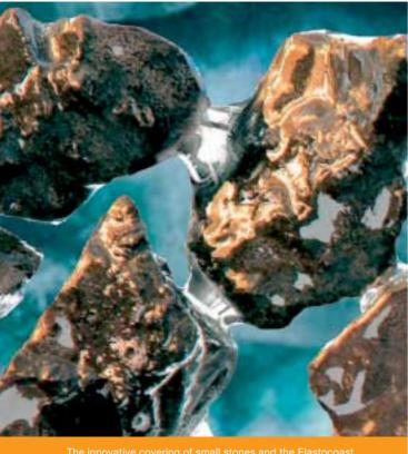
The innovative covering of small stones and the Elastocoast polyurethane system is elastic and porous. As a result, it car withstand the force of the water masses particularly well.
