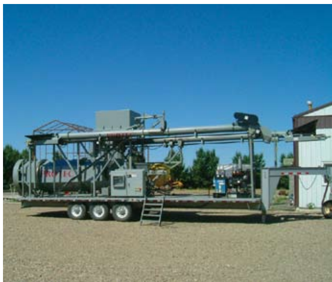
The Procoater, designed by ProCoat Technologies Inc., is a large scale seed treater capable of treating 1,100 bushels/hour of pulses and 1,650 bushels/hour of cereals and other crops.
