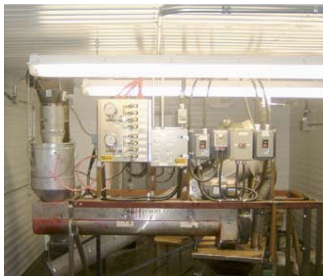
Westlock Seed Plant runs two of Graham Seed Treating Systems’ G3 units in parallel for increased capacity. The plant treats very high volumes of seed and speed is of the essence.
